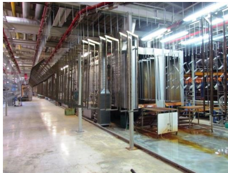
View of the pre-treatment plant at Kesseböhmer: The advantages of the optimised pre-treatment process are better adhesion of the paint, a reduction of the sludge and a working temperature that saves energy.
