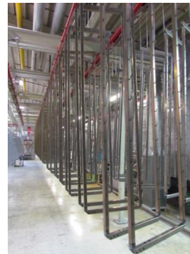
View of the pre-treatment plant at Kesseböhmer: The advantages of the optimised pre-treatment process are better adhesion of the paint, a reduction of the sludge and a working temperature that saves energy.
