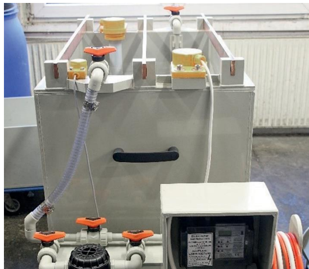
Figure 3: Tank for barrel tests directly at the plant. The tub is equipped with a pump, heating and ion exchange column.
