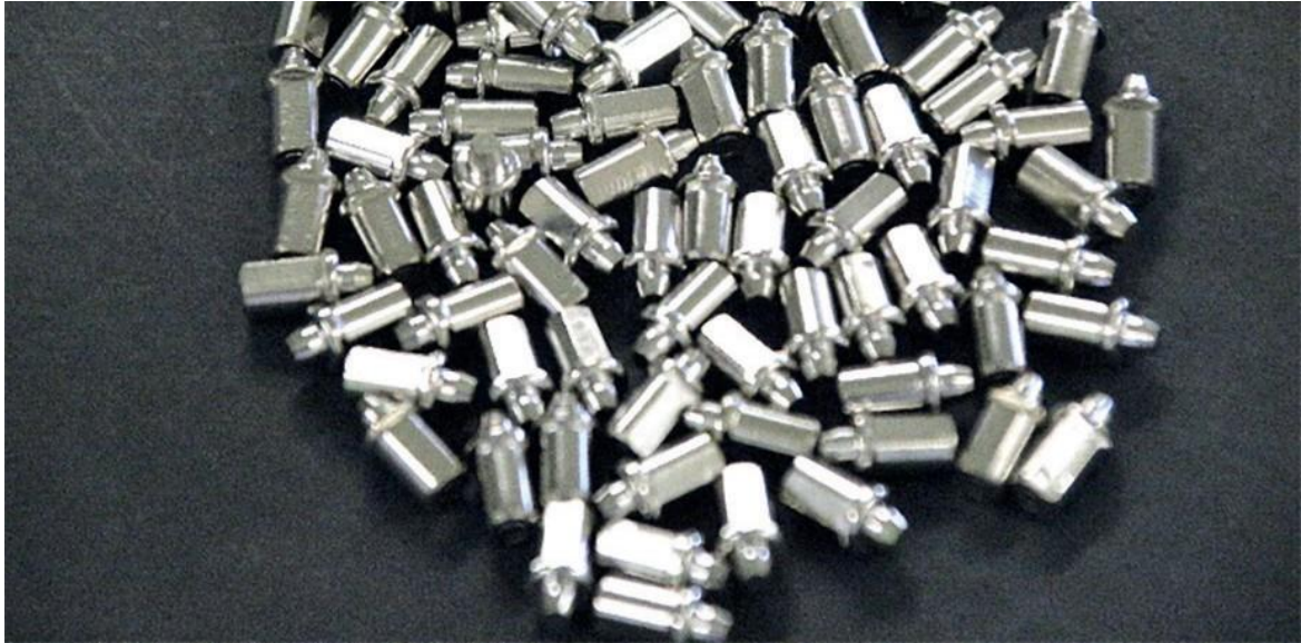
Figure 2: Coated samples at the customer (20 A, 30 min., 52 °C). A coating thickness of 0.18 - 0.29 µm could be measured.
