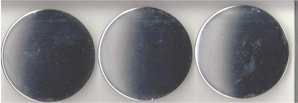
Samples after 96 h CASS test
