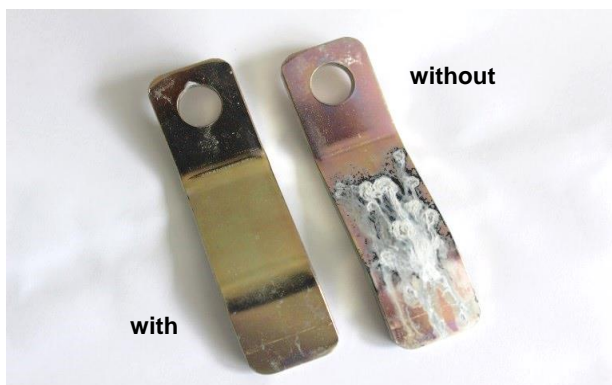
TOPAS 3100 + PROSEAL XZ 111 (+ PROSEAL Nanoadditiv) + SURFASEAL WL 150 after 840 h in DIN EN ISO 9227
