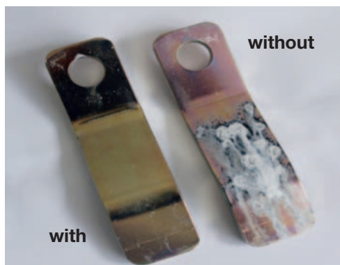
TOPAS 3100 + PROSEAL XZ 111 (+ PROSEAL Nanoadditiv) + SURFASEAL WL 150 after 840 h in DIN EN ISO 9227
